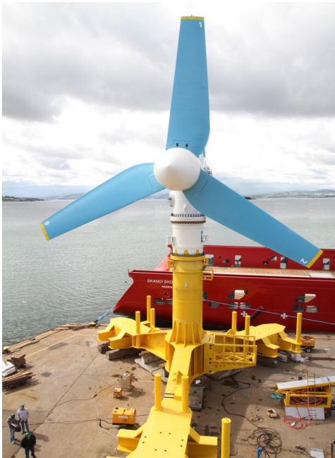
Final assembly test in the dry between turbine nacelle and test foundation
