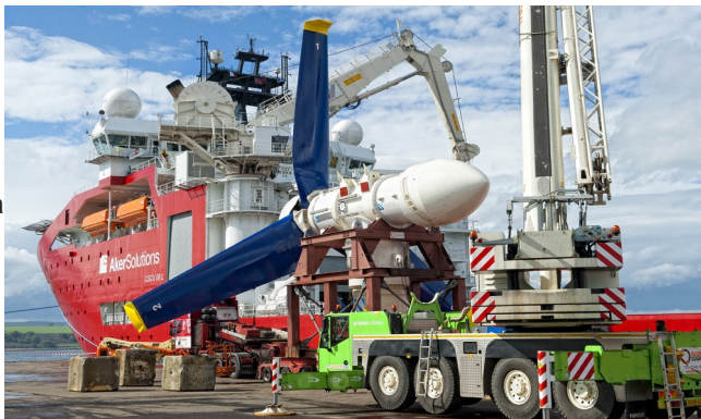
Atlantis 1MW AR1000 turbine prior to installation for open ocean testing at the European Marine Energy Centre (EMEC)
