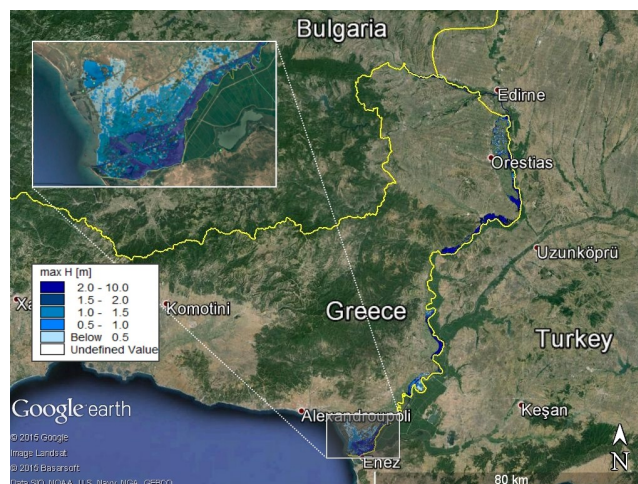
Basic scenario results of the Evros River and detail of delta inundation for 100 years recurrence interval. Data: SIO, NOAA, U.S. Navy, NGA, GEBCO ©2015 Basarasoft ©2015 Google.
