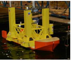
Testing the steel gravity structure transport in head sea. ©DHI
