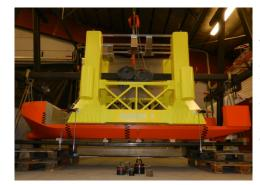
Joint heavy lift vessel and steel gravity structure model undergoing swing tests for transverse load characteristics. ©DHI Using a Qualisys tracking system, which tracks a number of reflective markers on the floating structure, we measured the overall motions. The marker tracks were converted to six degrees of freedom motions with respect to the centre of gravity as well as to other specified positions.
