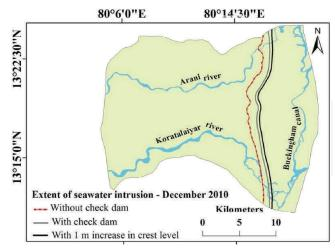
Extent of seawater intrusion without check dams, with existing check dams and with 1 m increase in crest level of existing check dams. © ANNA University/Rajaveni
