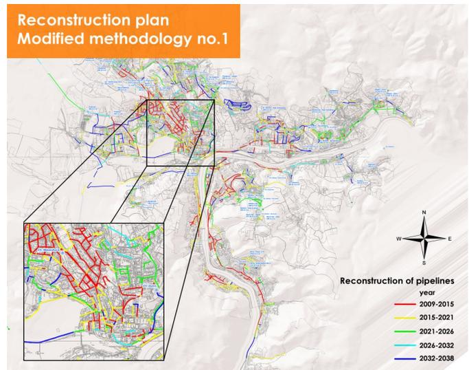
The water distribution system of Usti n/L, Czech Republic. The pipe network rehabilitation is part of the leakage management and is one of the most expensive tasks that the water utility needs to address. Advanced DHI modelling techniques help to prioritise and optimise investments.
