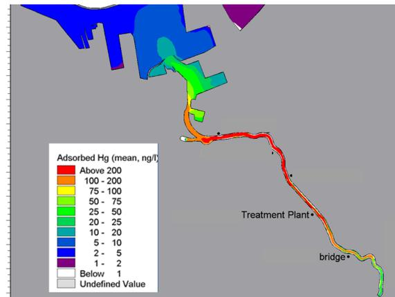
Modelling results from assessment of spreading of adsorbed Mercury in a river. Models can be used to predict future impacts or "hind-cast" spill events for compliance purposes.
