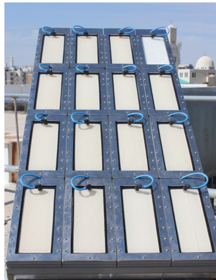
Photocatalytic membrane filtration pilot in Jordan © Inna Horovitz
