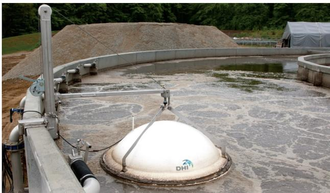
*During testing, the off-gas unit will be placed at the surface of the tank where the biological treatment process takes place. © DHI*
