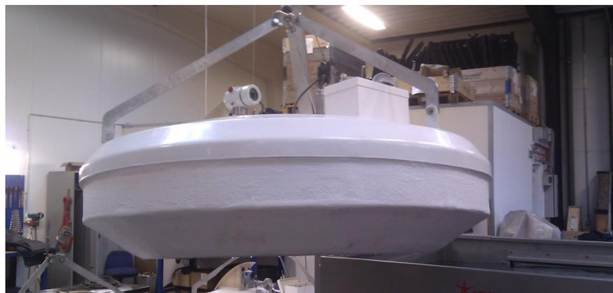
A specially designed off-gas unit is an essential part of the DHI monitoring unit for waste water treatment plants. ©DHI /Stjernholm
