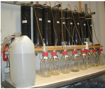
*We can perform numerous leaching tests and for a large number of different materials, such as waste, residues, soil, sediments, aggregates, construction products*
