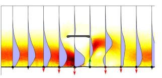
Shoreline evolution is based on a 2D sediment transport field. Changes in shoreline affects wave transformation, flow and the sediment transport. Source: Kristensen et al. (2013).
