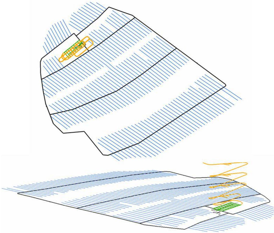
*Figure 7: Layout of the planned deep-rock repository in Forsmark that was implemented in MOUSE. The yellow line is the access ramp, extending from ground surface down to repository level (c. 450 m.b.s.l.). At repository level, green lines are tunnels and rock caverns in the central area, black lines are main and transport tunnels, and blue lines are so called deposition tunnels, from which deposition holes will be drilled.*
