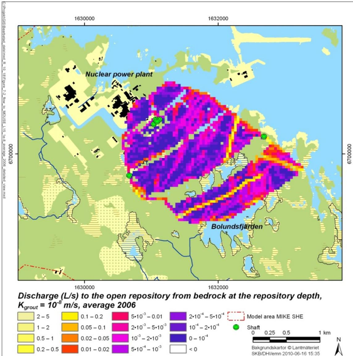
Figure 8: MIKE SHE-calculated annual average groundwater inflow (L/s) to the repository from each MIKE SHE grid cell at repository level (450 m.b.s.l., calculation layer 15) for grouting case B.
