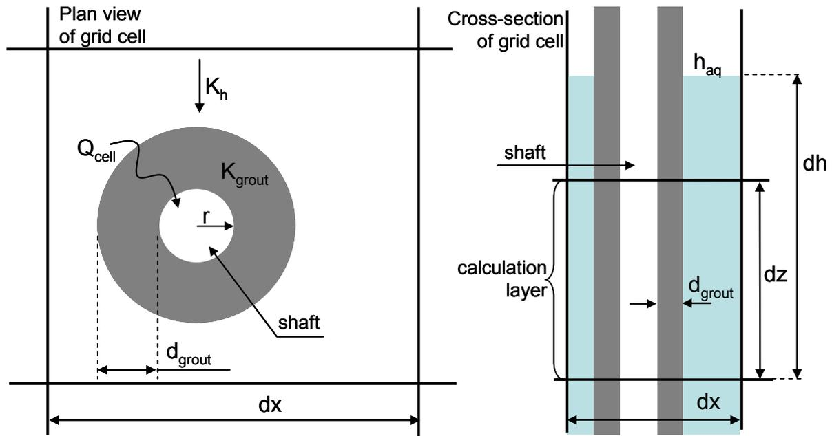
Figure 3: Calculation of groundwater inflow to a vertical cavity and associated parameters.
