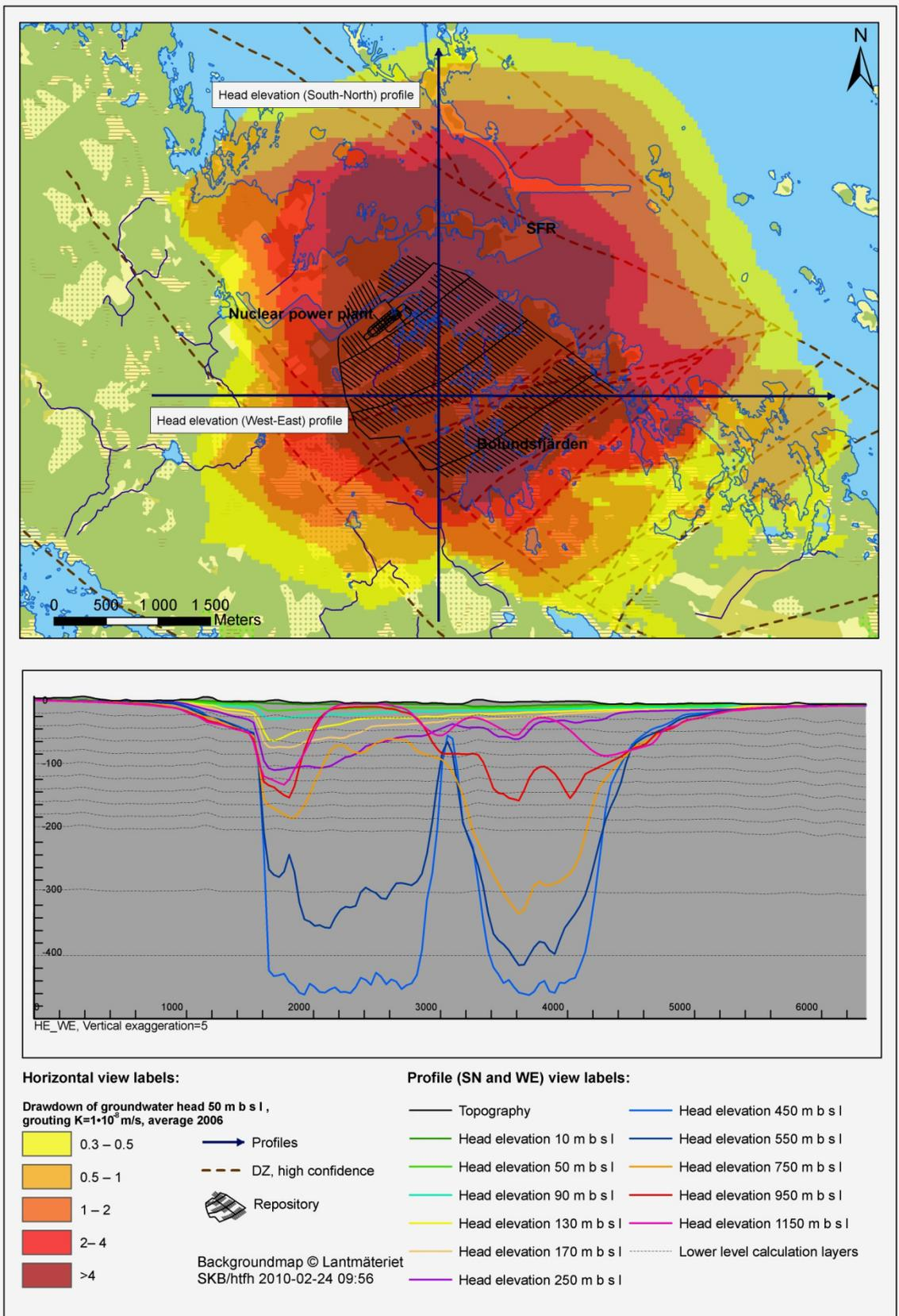
Figure 11: MIKE SHE-calculated annual average hydraulic heads in different calculation layers (coloured lines) along a west-to-east profile across the model area and the repository. The geographical location of the profile is shown in the upper map, which also shows the calculated hydraulic-head drawdown in the rock at the level 50 m.b.s.l. The results refer to grouting case B.
