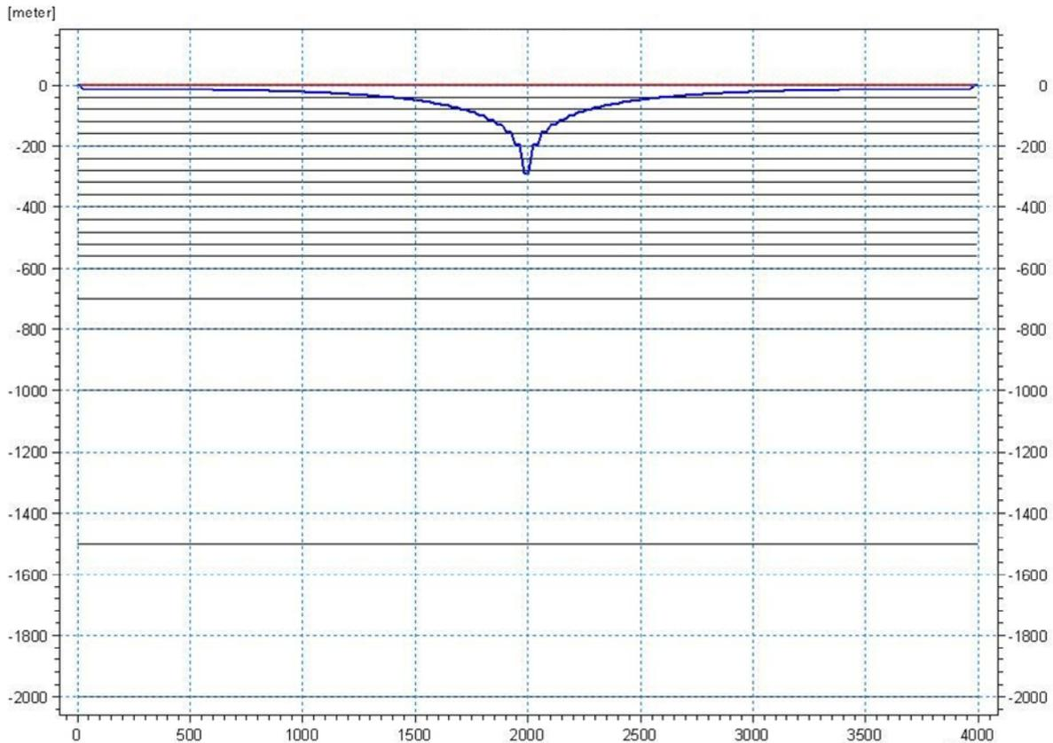
Figure 4: Cross-section of the MIKE SHE test-model setup. At the top boundary ( $z = 0$ ) the hydraulic head is fixed at 0 m. The horizontal black lines show the lower level of each MIKE SHE calculation layer. The blue line represents the calculated hydraulic head in the layer where the hypothetical tunnel is located (tunnel centre at  $z = -500$  m) for one of the simulation cases.
