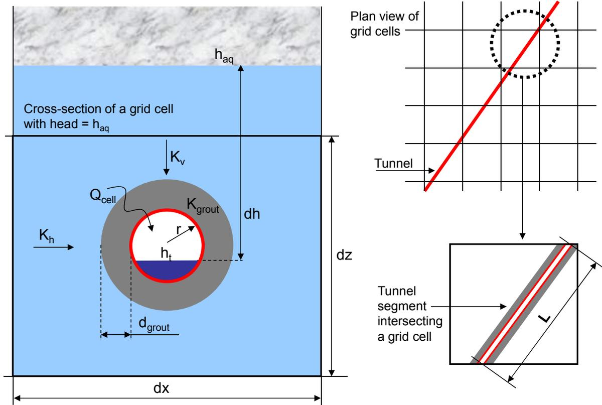
Figure 2: Illustration of the new MIKE SHE-MOUSE coupling routine ( $MS-M_{\text{new}}$ ) and associated parameters.
