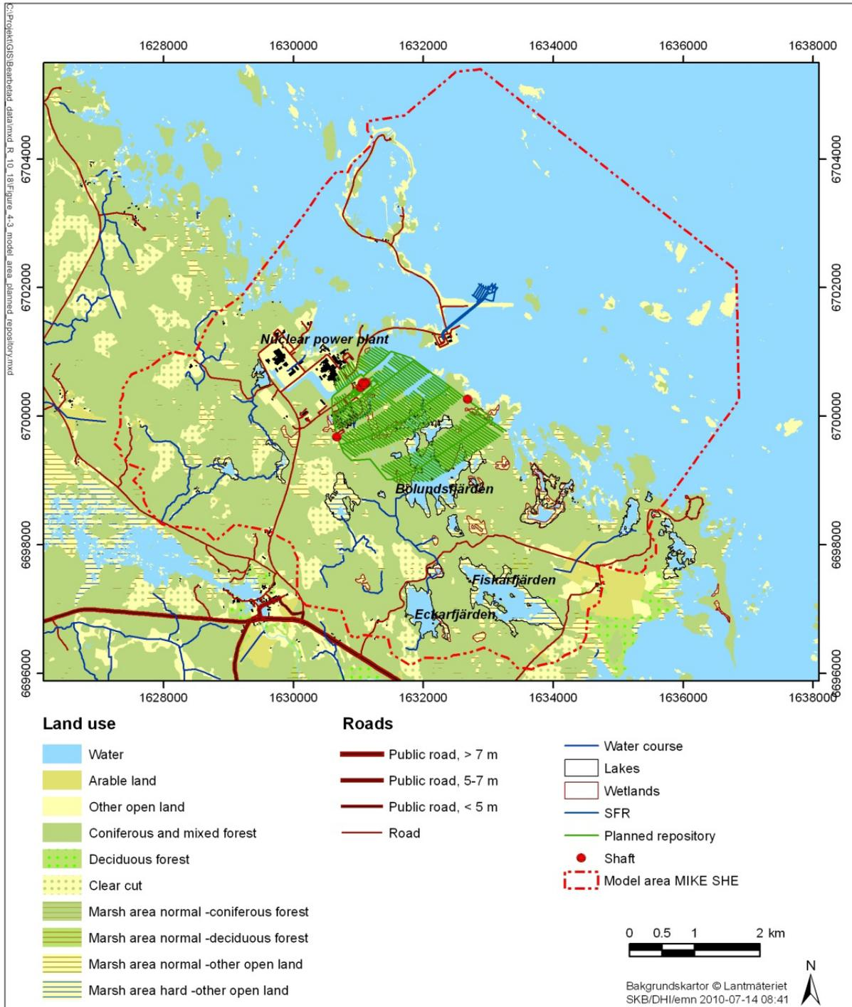
Figure 6: The Forsmark MIKE SHE model area and the layout of the planned deep-rock repository (layout D2, version 1.0).
