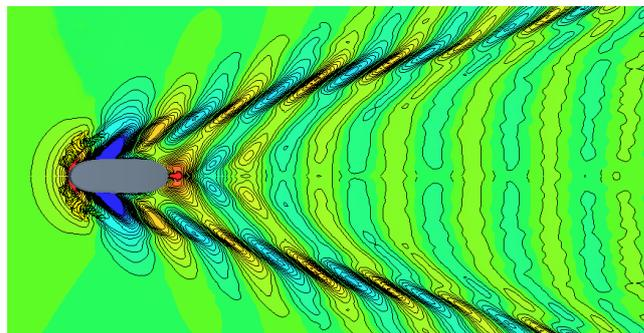
Waves generated by a tug calculated using Computational Fluid Dynamics.
