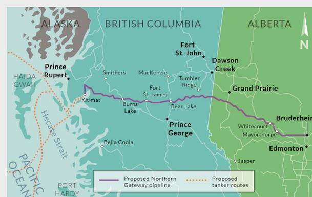
The planned project consists of two parallel pipelines between an inland terminal at Bruderheim, Alberta, and a marine terminal near Kitimat, British Columbia, each with a length of 1,177 km. The Kitimat terminal will comprise two tanker berth platforms, one serving Very Large Crude Carriers and another serving Suezmax-type condensate tankers. For more information about this project, please refer to <http://www.gatewayfacts.ca/>.
