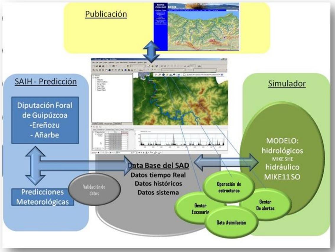
Figure 11: Architecture of the DSS system
