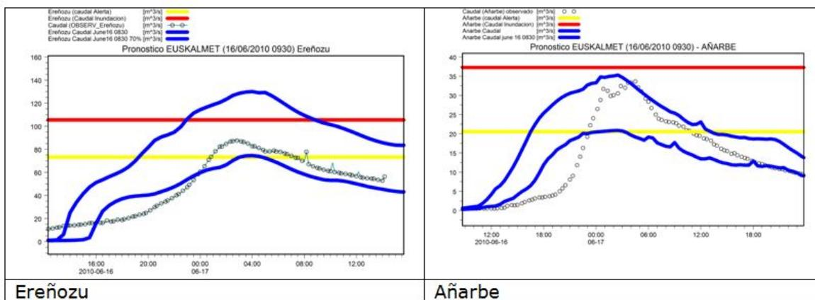
Figure 20 Forecasted and observed discharge and the Añarbe measuring station
