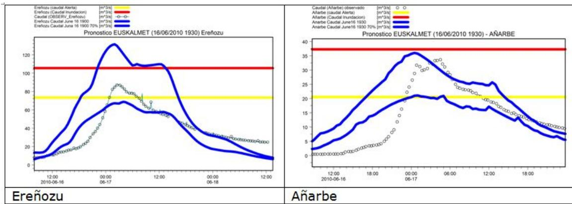
Figure 21: Forecasted and observed discharge and the Ereñozu and Añarbe measuring stations
