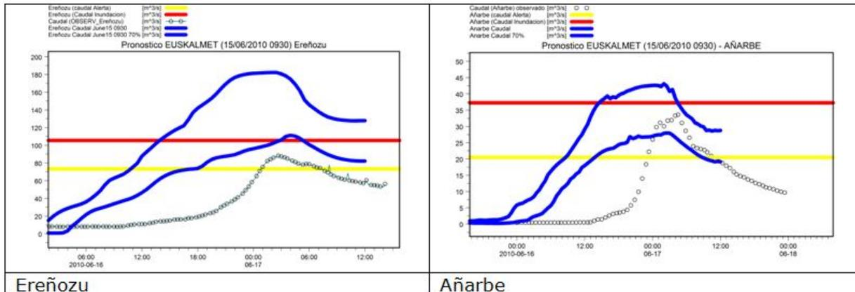
Figure 18: Forecasted and observed discharge and the Ereñozu measuring station
