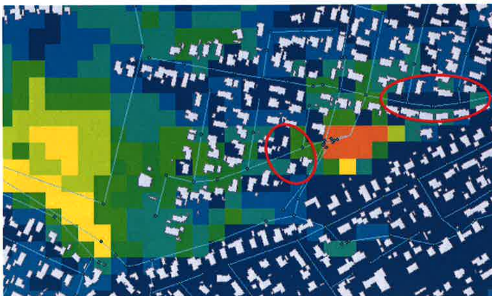
Figure 82. High elevations blocking flow paths due to interpolation of topography grid into bigger grid size (showing real shapes for structures)
