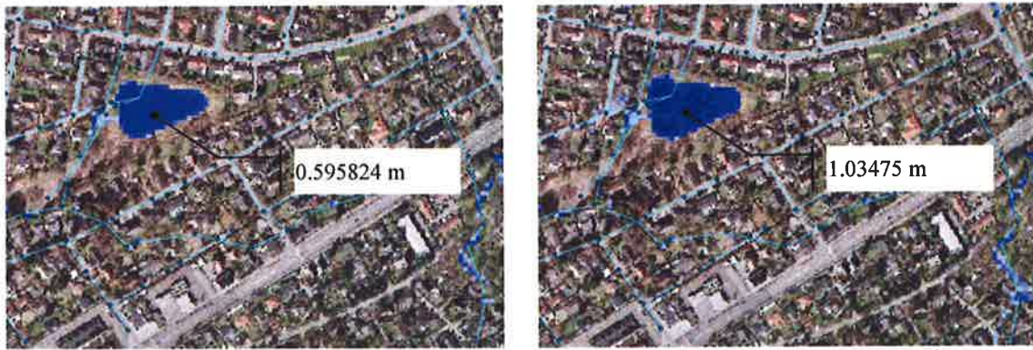
(a) Before MOUSE basin removal (b) After MOUSE basin removal Figure 62. Water depth in a topographical basin before (a) and after (b) basins were removed in MOUSE
