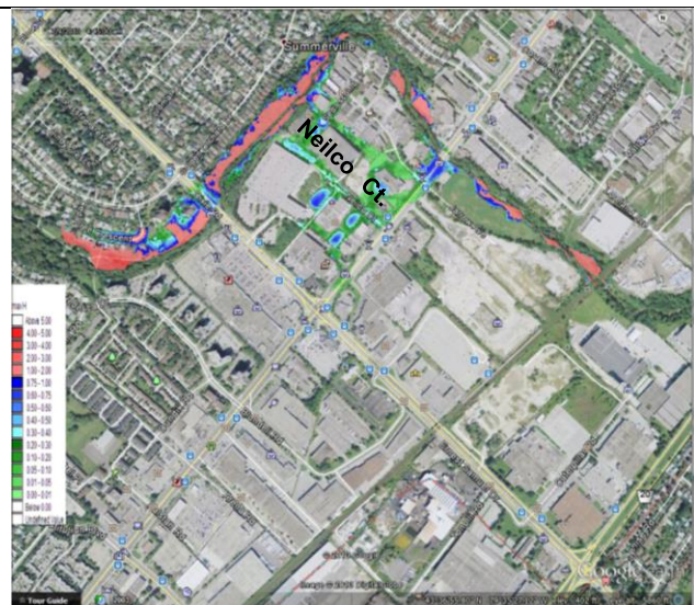
Figure 8: Maximum flood extent and flood depth with no spilling west of Neilco Court
