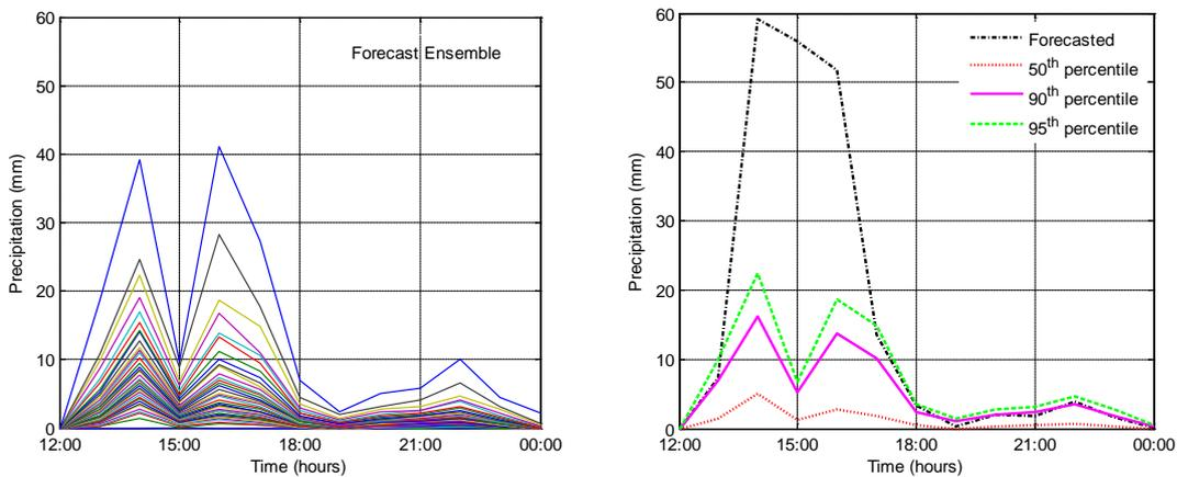
Figure 3: Forecast ensemble from probabilistic rainfall model, forecasted 12-hour rainfall and forecast percentiles estimated from the forecast ensemble
