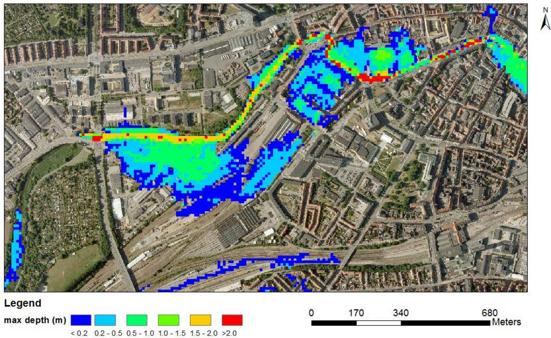
Figure 7: Maximum depth obtained when using the 95<sup>th</sup> percentile of the rainfall probability distribution (direct quantile approach)
