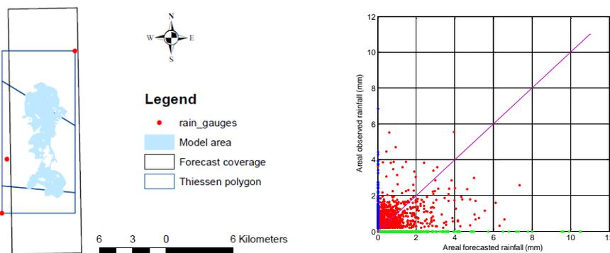
Figure 1: Left: Model area, total forecast area used, Thiessen polygons and rain gauge locations. Right: observed and forecasted hourly areal rainfall for a forecast lead time of 12 hours.
