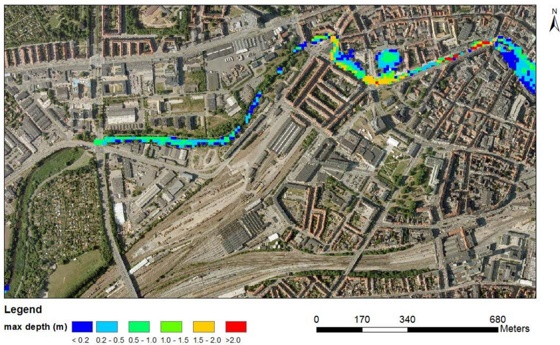
Figure 4: 50<sup>th</sup> Percentile of the maximum flood depths obtained from the rainfall ensembles (LHS approach)
