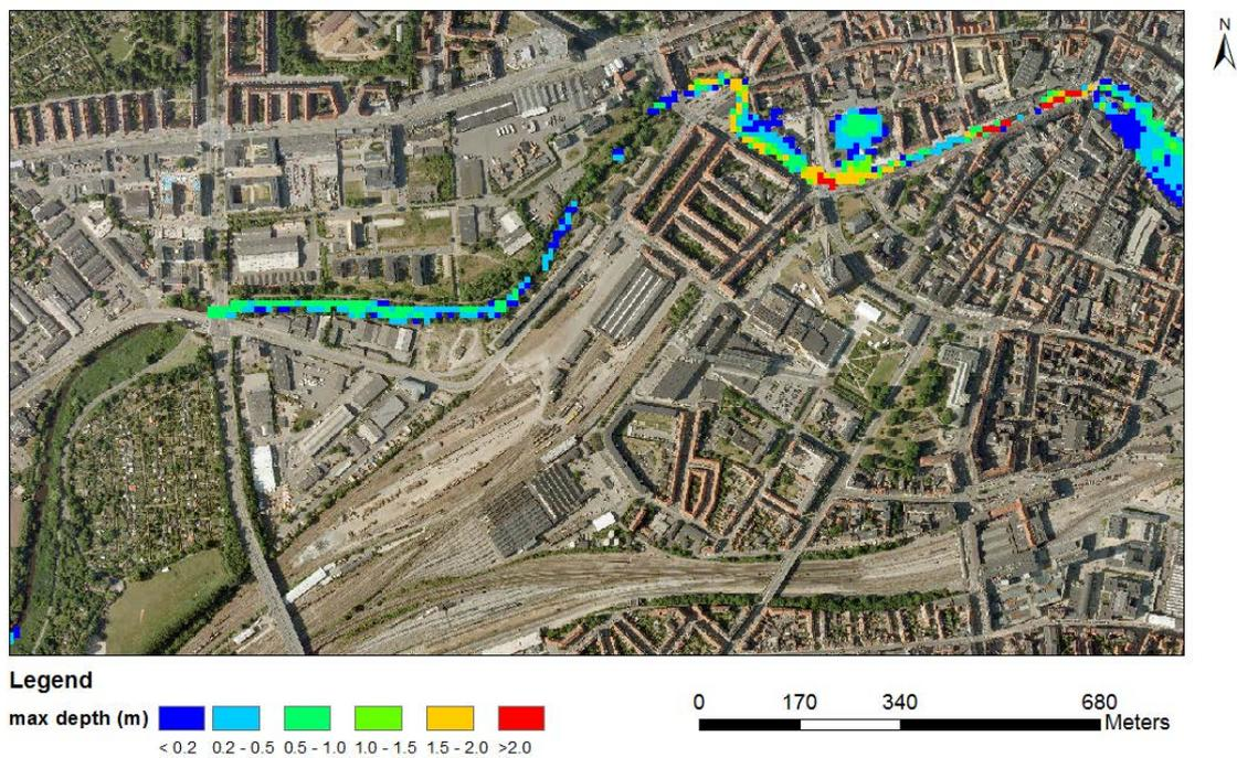
Figure 5: Maximum depth obtained when using the 50<sup>th</sup> percentile of the rainfall probability distribution (direct quantile approach)
