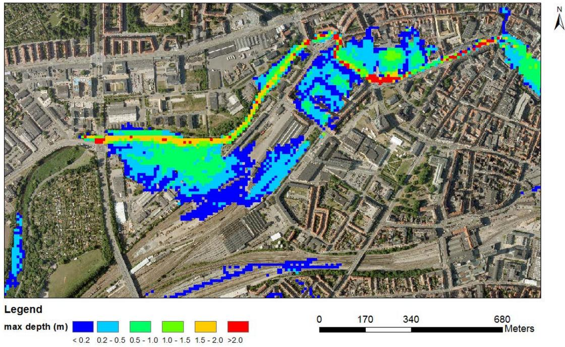
Figure 6: 95<sup>th</sup> Percentile of the maximum flood depths obtained from the rainfall ensembles (LHS approach)
