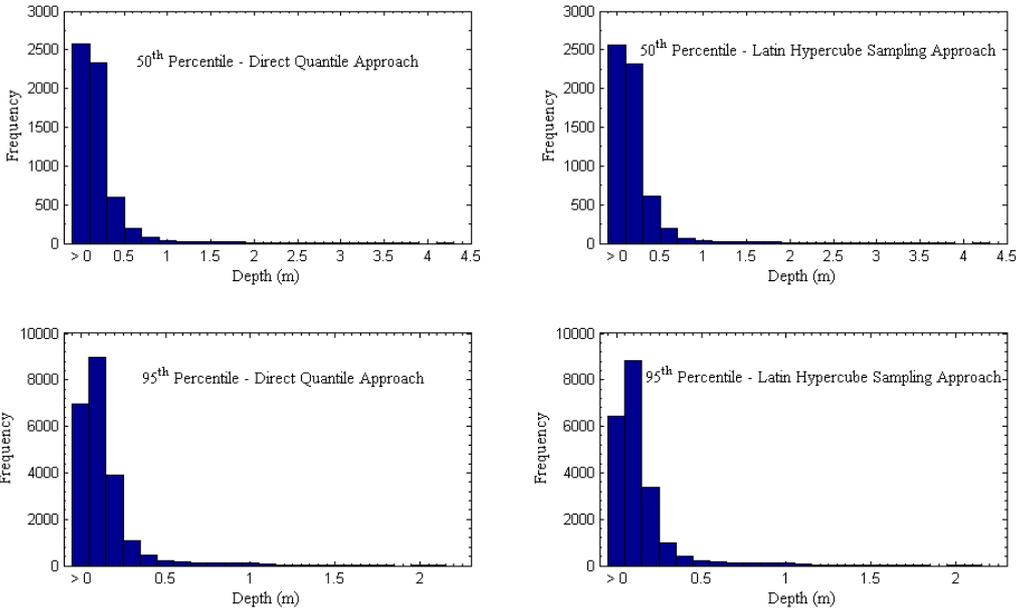
Figure 8: Comparison of the 50<sup>th</sup> and 95<sup>th</sup> percentile of the maximum flood depth obtained using the direct quantile approach and the Latin hypercube sampling approach. The data represents the maximum flood depth obtained for each grid cell over the model domain
