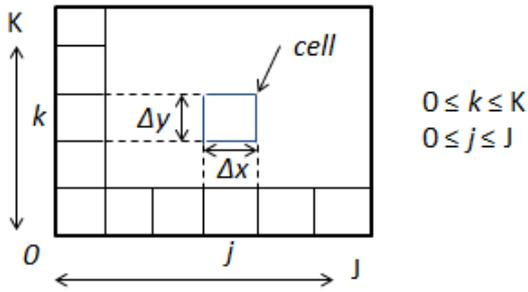
Figure 2: Schematic representation of 2D computational domain for the 2D overland model
