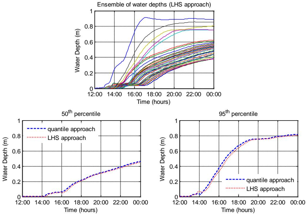
Figure 10: Comparison of time series of water level at a selected location in the urban flood model
