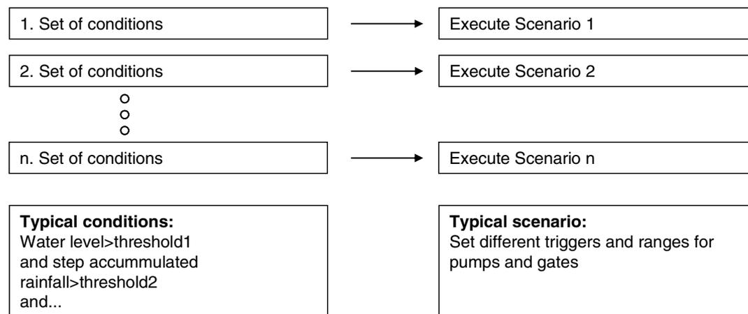
**Figure 5 Selection and execution of appropriate flood forecasting model scenario based on a set of physical conditions in the hydrological and hydraulic system**
