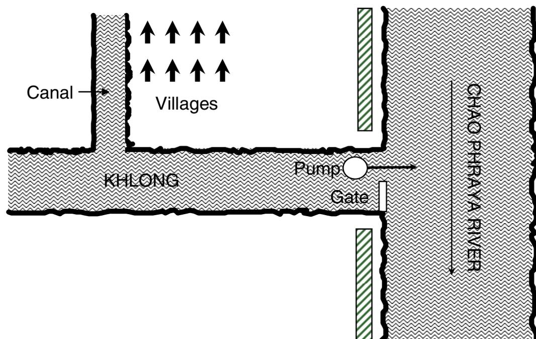
**Figure 4 Typical layout of hydraulic structures in the centre of Bangkok**
