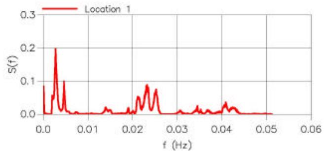
Fig 4 Example of calculated wave spectrum of the white noise signal in the Multipurpose Basin.
