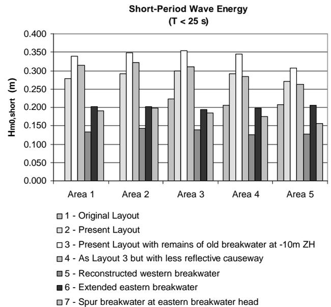
Fig 9 Comparison of average short-period ( $T < 25s$ ) wave disturbance coefficients in areas 1 to 5.
