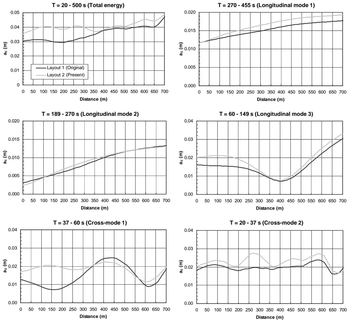
Fig 7 Comparison of long wave energy ( $a_c$ ) in Layouts 1 and 2 for the different oscillation modes
