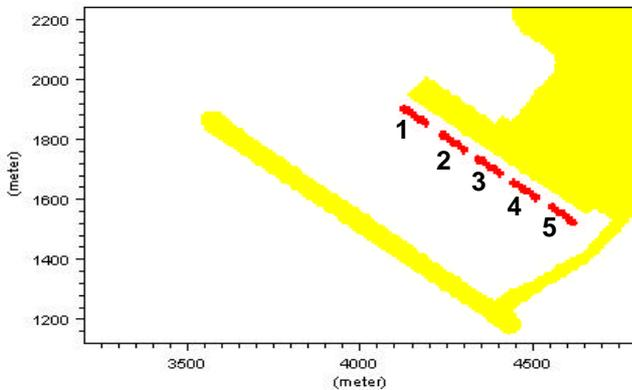
Fig 8 Extraction areas for average wave disturbance coefficients ( $k$ ).
