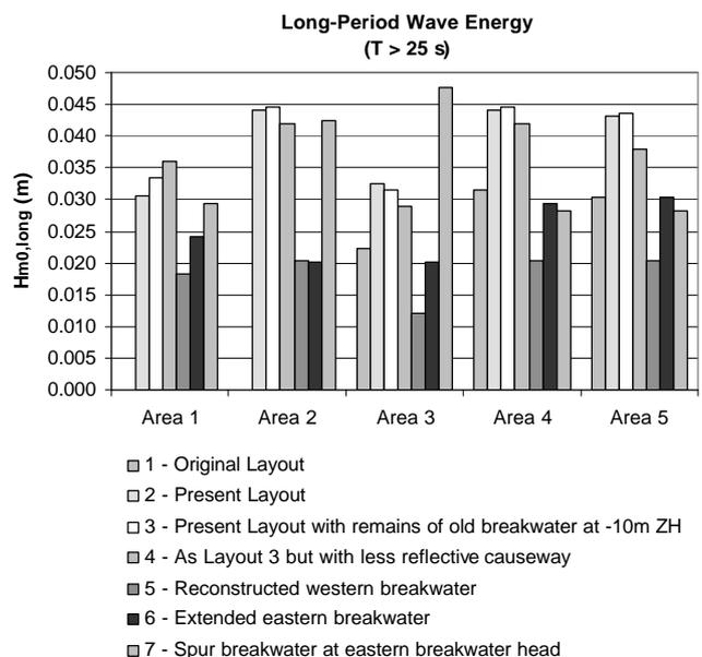
Fig 10 Comparison of average long-period ( $T > 25s$ ) wave disturbance coefficients in areas 1 to 5.
