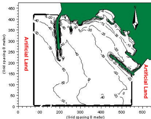
Fig 2 Applied model bathymetry (present conditions)
