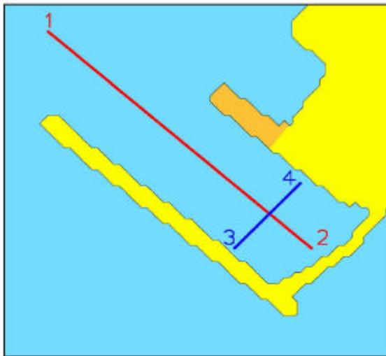
Fig 5 Extraction lines for surface elevation envelopes in the different frequency bands.
