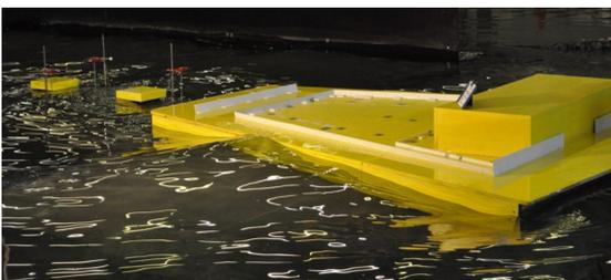
Testing a protective layout consisting of wave screens at our physical test facility.
