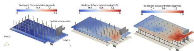
Plots of the free surface with sediment concentration for three stages of the filling of the retention basin at 500 seconds (left), 4,000 seconds (middle) and 8,500 seconds (right). ©DHI
