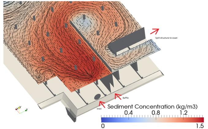
Close up of contour plot near the free surface for the model with a baffle included. The model has been spilling for 500 seconds. Surface vectors and streamlines show the location of the attachment of the inflow jet as well as the flow path around the baffle to the spill outlets. © DHI
