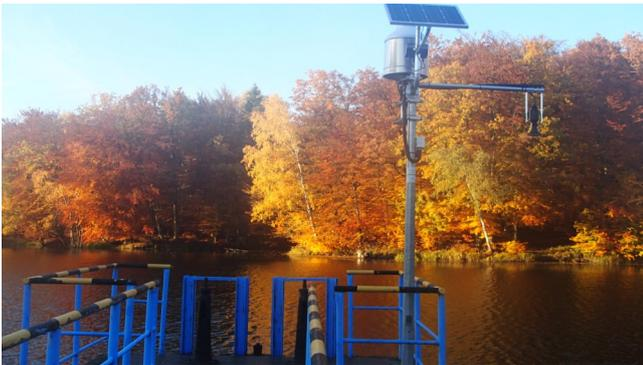
Telemetric station for hydrological and meteorological measurements.
