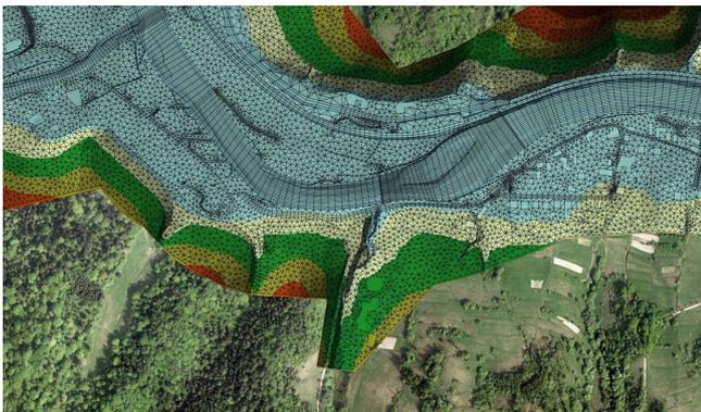
Flexible Mesh with Topography of the terrain © DHI
