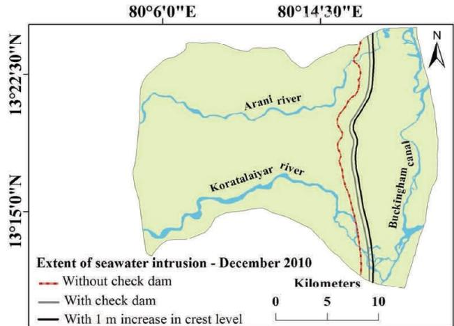
Extent of seawater intrusion without check dams, with existing check dams and with 1 m increase in crest level of existing check dams. © ANNA University/Rajaveni
