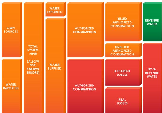
Some of the possible various components building up the structure of a Water Audit, following the IWA/AWWA-methodology (adjusted). Within these components, water volumes are tracked, revealing weak spots and losses.
