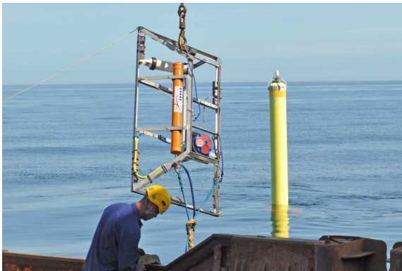
Lowering the current/wave meter during deployment of the buoy. The floating buoy can be seen in the background.
