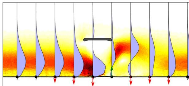
Shoreline evolution is based on a 2D sediment transport field. Changes in shoreline affects wave transformation, flow and the sediment transport. Source: Kristensen et al. (2013).
