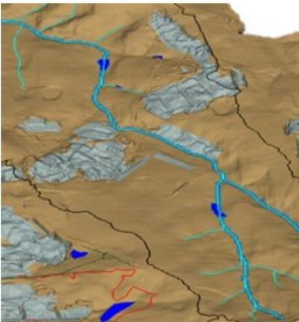
*Mine hydrology model layout showing affected areas in the mine within a catchment context (highlighted in grey)*
