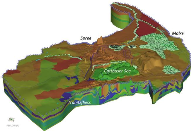
Overview of FEFLOW 3D groundwater model with applied conductivities and boundary conditions
