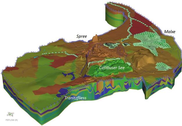
Overview of FEFLOW 3D groundwater model with applied conductivities and boundary conditions. © DHI
