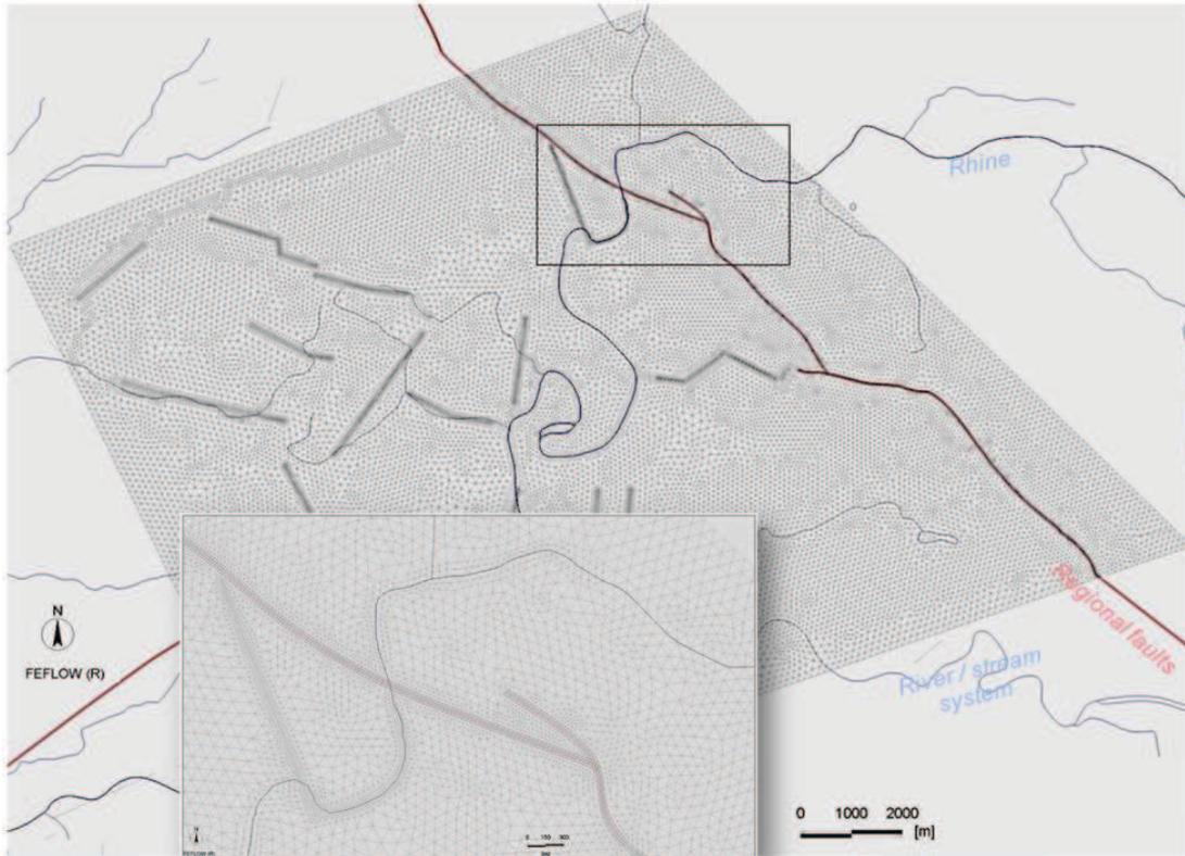
a) Finite-element mesh local model ZNO-SR with detailed view
