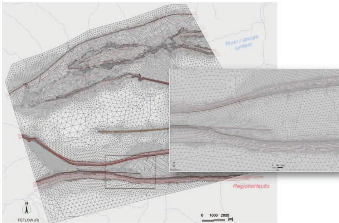
b) Finite-element mesh local model JS with detailed view
