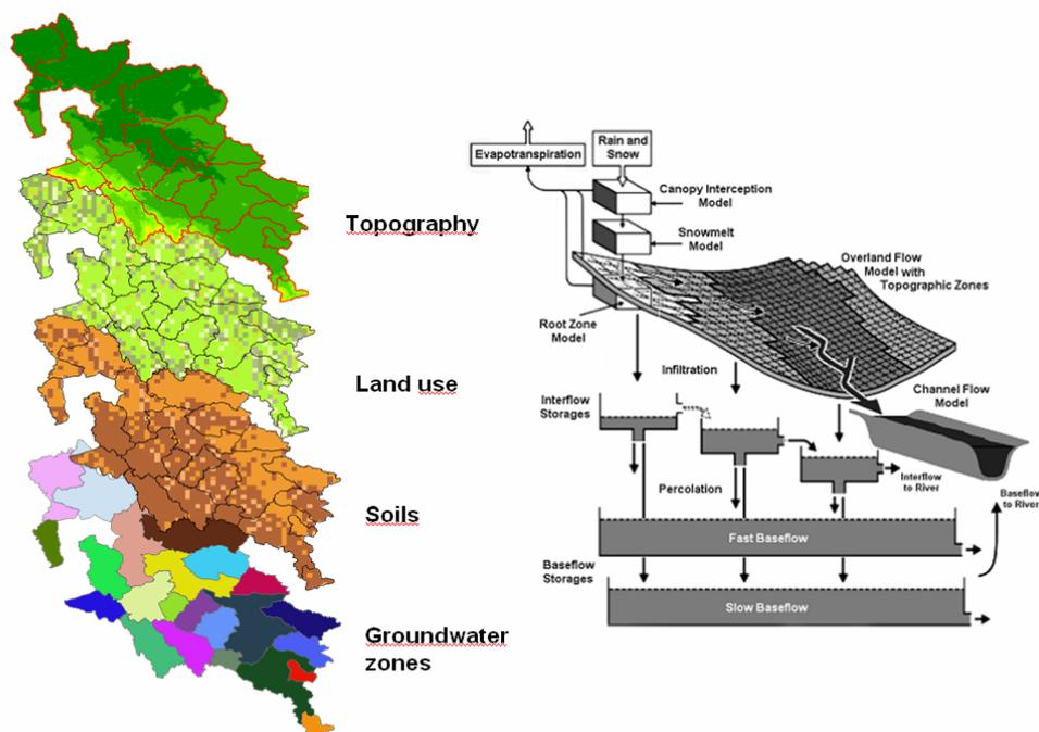
Figure 6 Left figure: The spatial input data and subcatchments used to treat the spatially distributed data. Right figure the conceptual process representation for subcatchment-based rainfall-runoff modelling.
