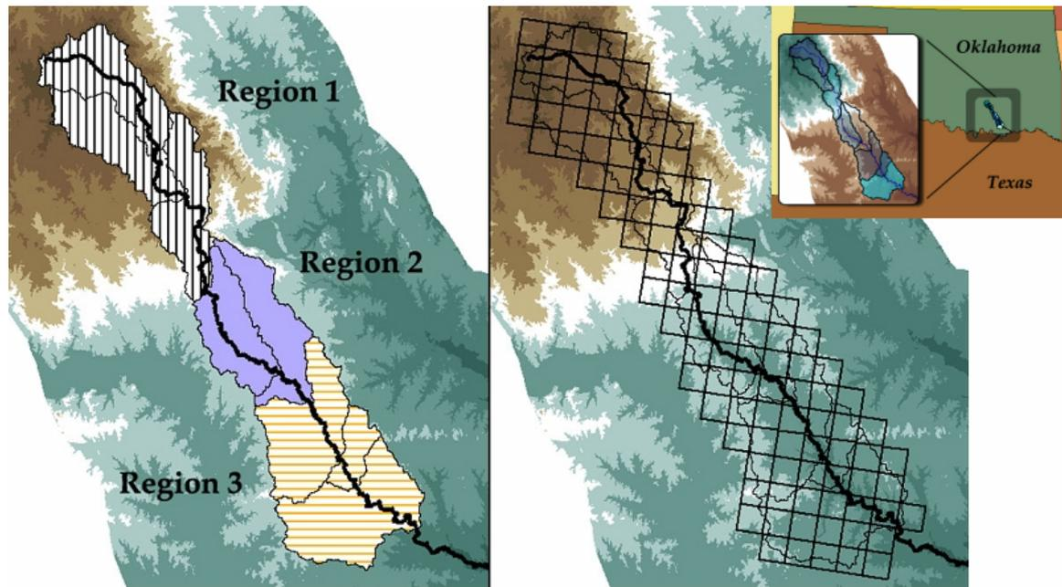
Figure 2 Different spatial discretizations were used to model the Blue River. The figure on the left shows the 8 subcatchments used in conceptual modelling and the parameter regions used for calibration. The figure on the right shows the 4-km NEXRAD grid used for the grid-based modelling. Inset: Location of the Blue River catchment
