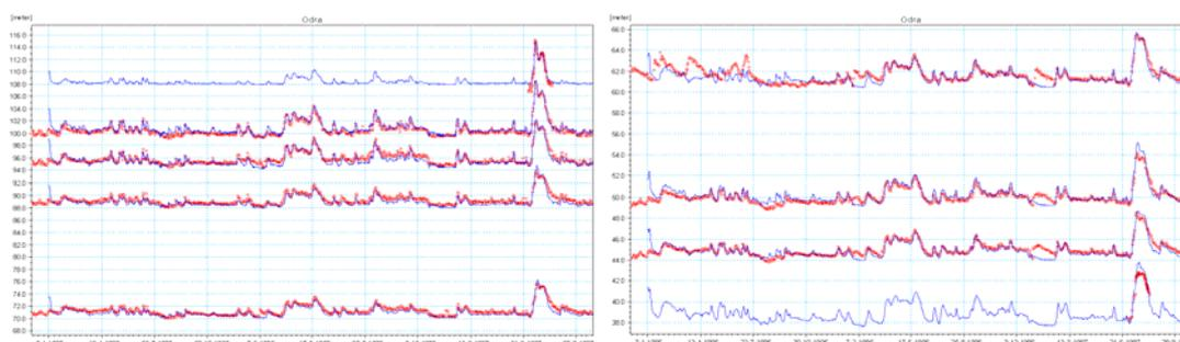
Figure 5 Comparison of the measured (symbols) and simulated (line) water levels from the river model calibration, 1995-1997 along the main river system.
