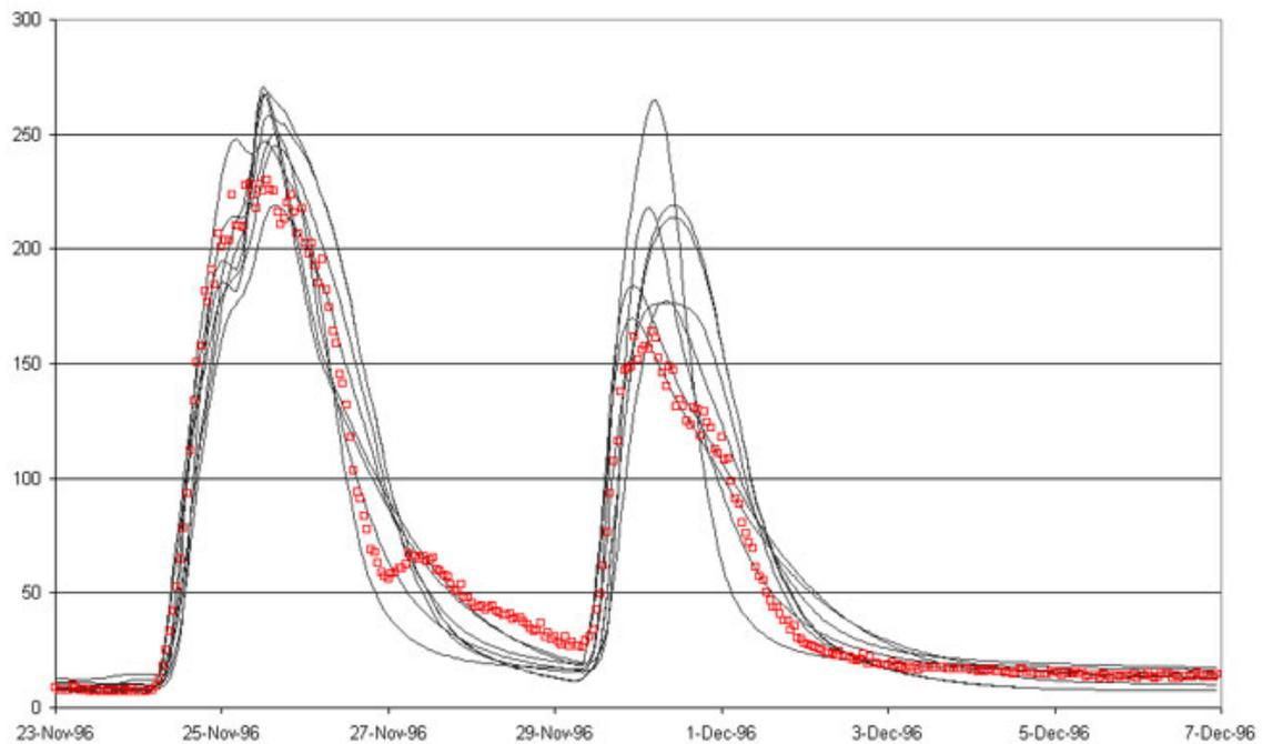
Figure 3 Two flood events in the Blue River Basin, The symbols show the observed flows and the solid lines the predicts using 10 different calibrated models (Butts et al., 2004a&b)
