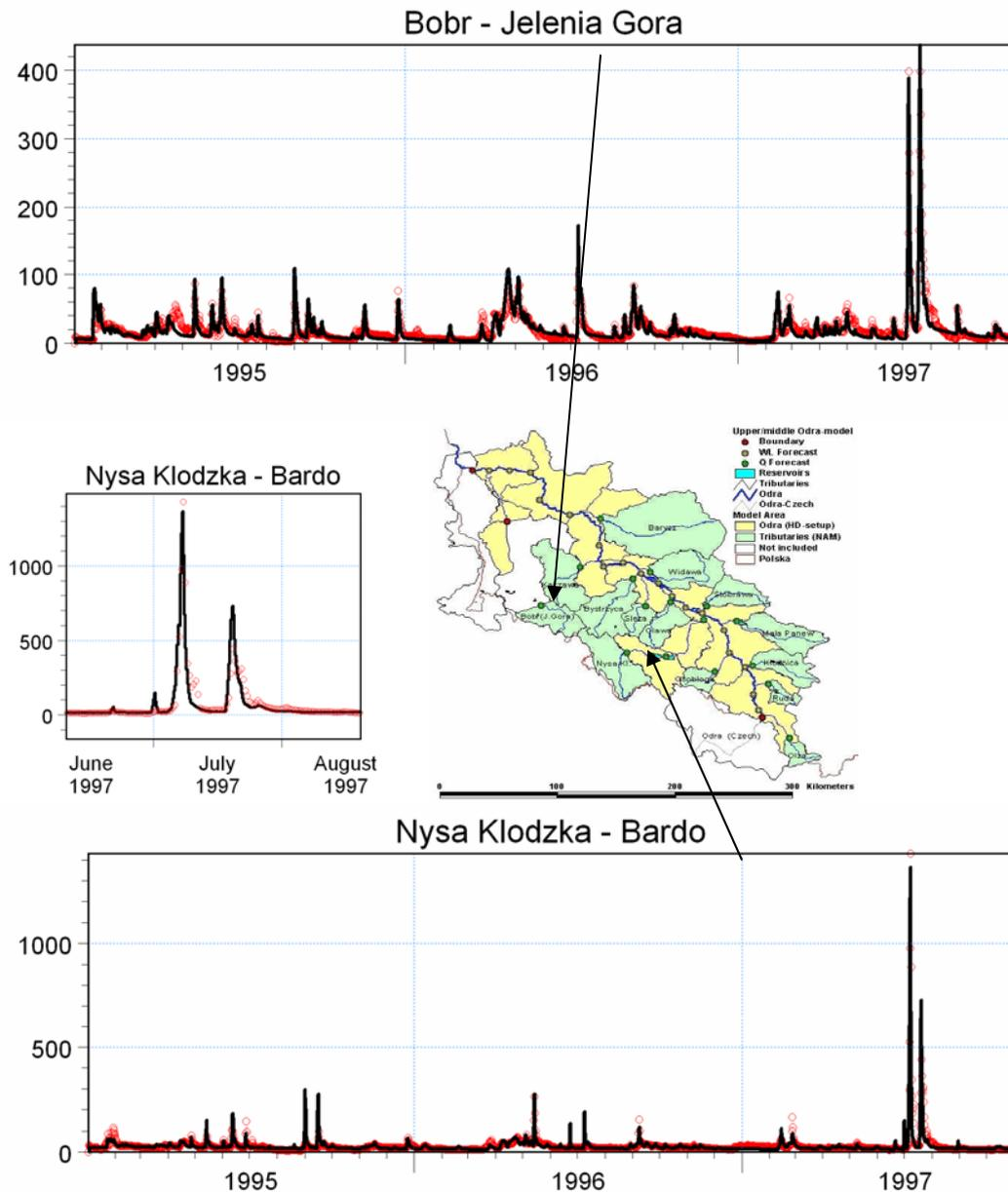
Figure 7 Spatial comparison of the measured (symbols) and simulated (line) discharges for the Bardo station on the Nysa Klodzka river and the Jelenia Gora station on the Bobr river
