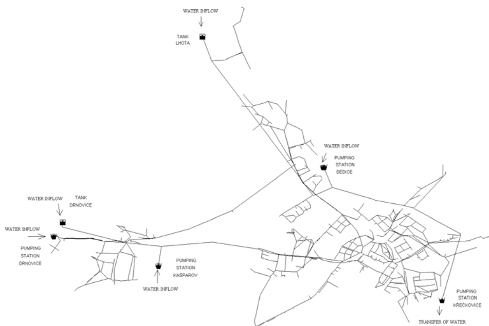
Fig.1. Computational scheme of the water supply network of Vyškov - ODULA modelling package
