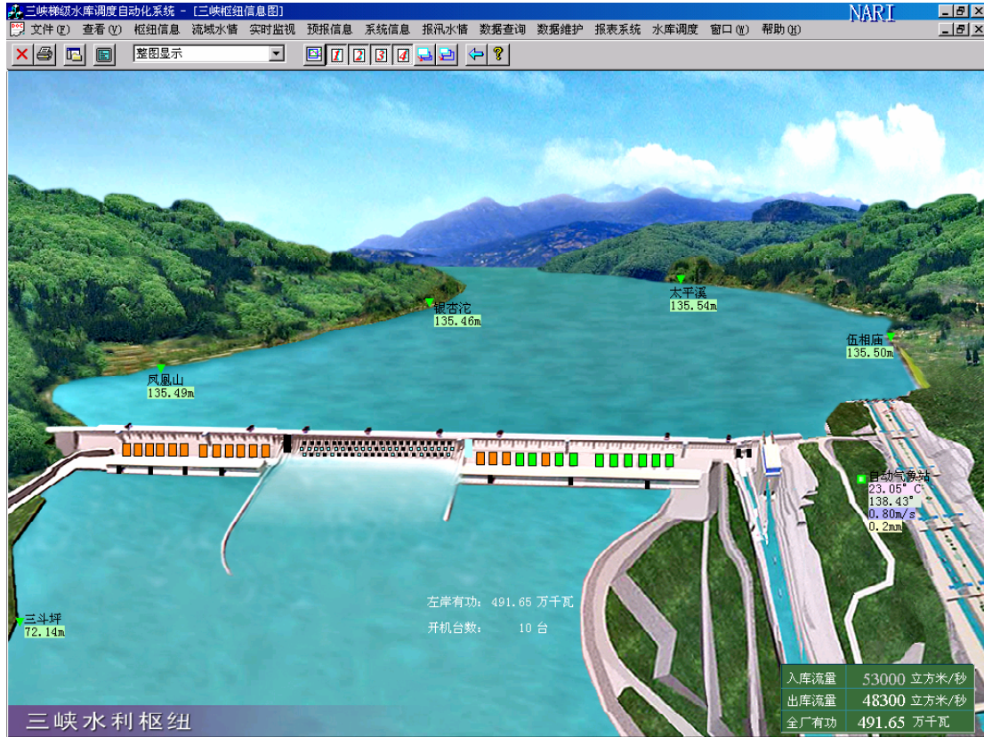
Figure 4 – Three Gorges Dam. The spillways are located in the middle of the dam, the flushing gates at the bottom and the ship locks to the right. The turbines are depicted as rectangular units.
