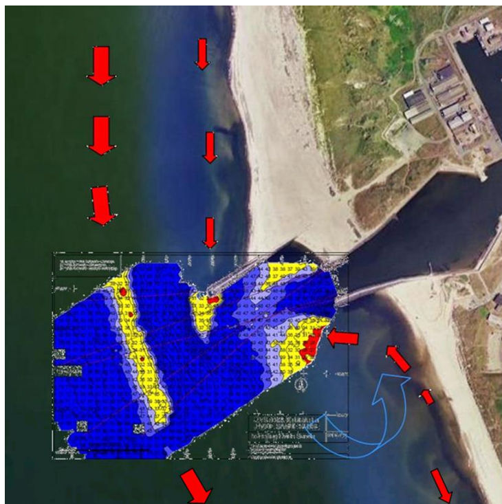
Figure 4: Typical bathymetric survey of the access channel superimposed on an aerial view of Hvide Sande harbour; the yellow colour shows depths between 3 and 4 m, red shows depths less than 3 m. The red arrows illustrate the sediment transport pattern and the blue arrow the circulation pattern in the lee of the harbour
