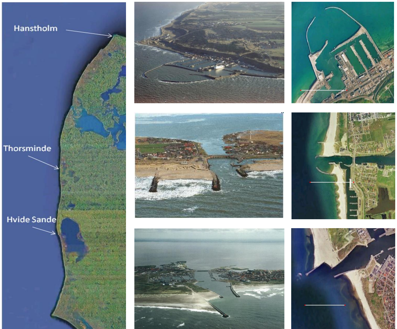
Figure 1: Left: Location map of bypass harbours. Middle: Aerial photos. Right: Satellite images (approx. same scale, line = 500 m). Thorsminde (old layout at aerial photo and new layout at satellite image) and Hvide Sande Harbours at a straight coast and Hansthholm at a headland
