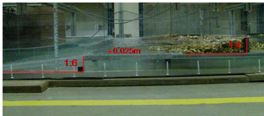
Figure 4.2: The harbor's bed and bathymetry.
