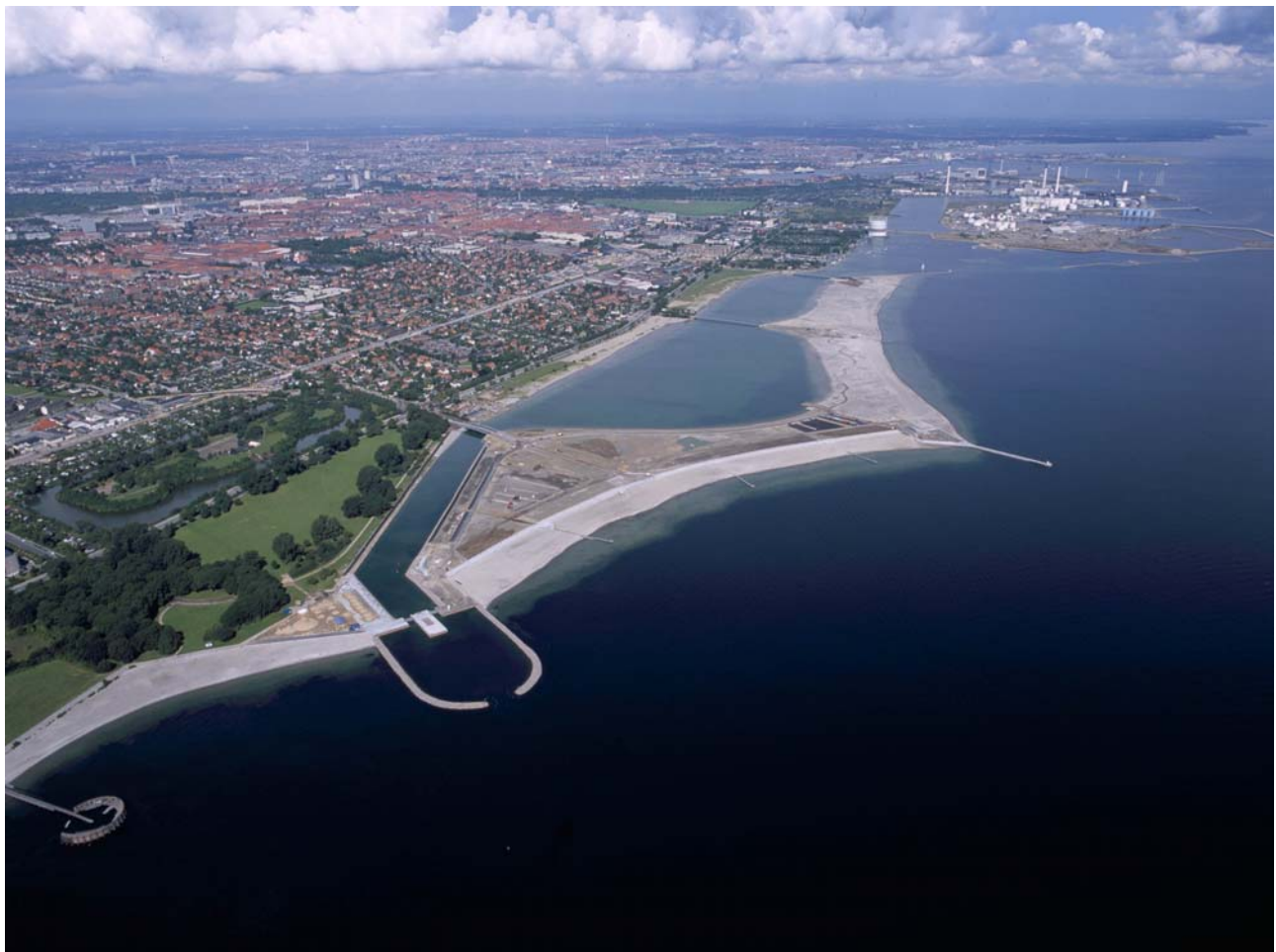
Figure 12. Aerial photo of Amager Beach Park, which consists of the following main elements: island with terminal structures north and south and a separating headland between northern and southern beaches and a lagoon.
