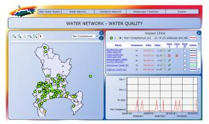
User interface of DHI's water management system. Numerous menus offer information on the water balance, water quality, status of dams, wastewater quality compliance, etc. The current pane displays various water quality parameters within the water network, such as the number of coliform bacteria, aluminium concentration and others.
