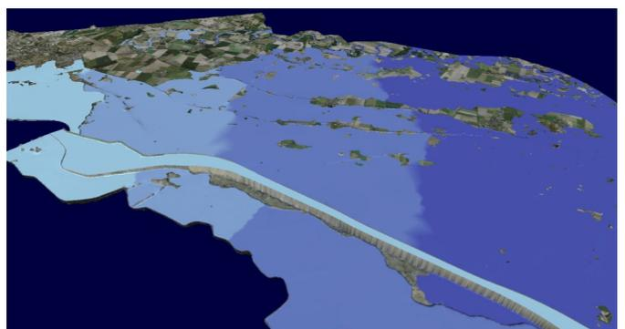
Range of flooded area (1,000 year return period discharge). Digital Terrain Model and Orthophotomap © Eurosense s.r.o. / Geodis Slovakia s.r.o. 2008-2011.
