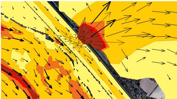
Detail of the current speed map with vectors showing flow direction (1,000 year return period discharge). Digital Terrain Model and Orthophotomap © Eurosense s.r.o. / Geodis Slovakia s.r.o. 2008-2011.
