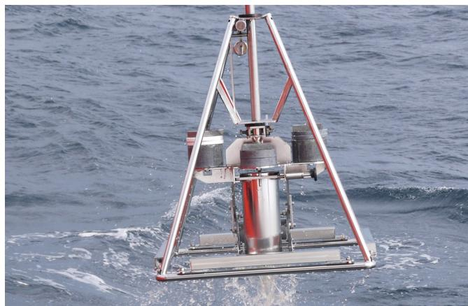
*Sediment samples being collected around platforms using a HAPS core sampler.*
