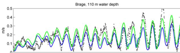
*Illustration of improvement of current speeds when implementing cut-cells and optimising transition depth. Black dots show measurements, while the blue line and the green line show model results before and after model improvements, respectively.*
