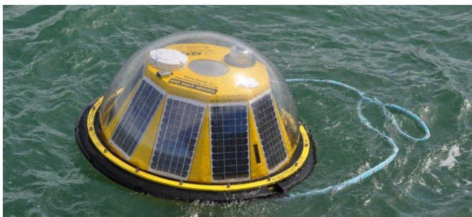
One of the wave buoys which provides on-line data and supports the hydro-dynamic model.
